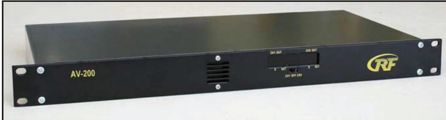
AV-200T is designed for modulating analogue video and stereo audio to COFDM signal.
