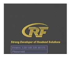
At power-up this welcome screen is displayed. Main SW and user interface SW version numbers plus unit serial number are shown.
