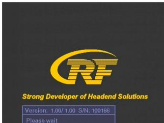
At power-up this welcome screen is displayed. Main SW and user interface SW version numbers plus unit serial number are shown.
