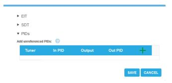
→ Under **Add unreferenced PIDs**, click the green plus sign in the table header. A line for entering the PID is inserted.
