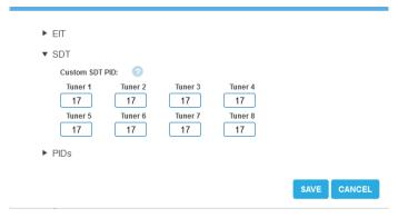
→ For tuners 1 to 8 or 16, enter the PIDs used to transmit the SDT. Permissible values are 32 to 8190. The entered PID of the SDT is then converted to PID 17.
