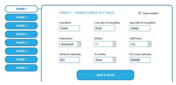
The SAT IF frequency of the transponder is entered in the input field **Freq (MHz)**.
