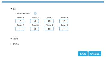
→ For tuners 1 to 8 or 16, enter the PIDs used to transmit the EIT. The entered PID of the EIT is then converted to PID 18.
